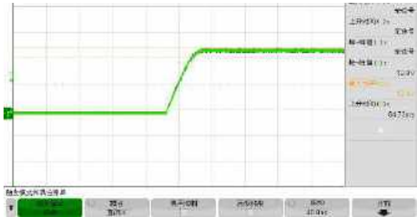
Figure 6, Output voltage established (Iout = 20A)
