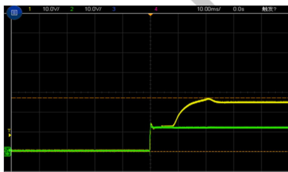
Figure 6, Output voltage established (Iout = 3A)
