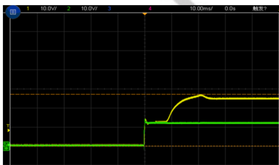
Figure 6, Output voltage established ( I_{out} = 1\text{A} )
