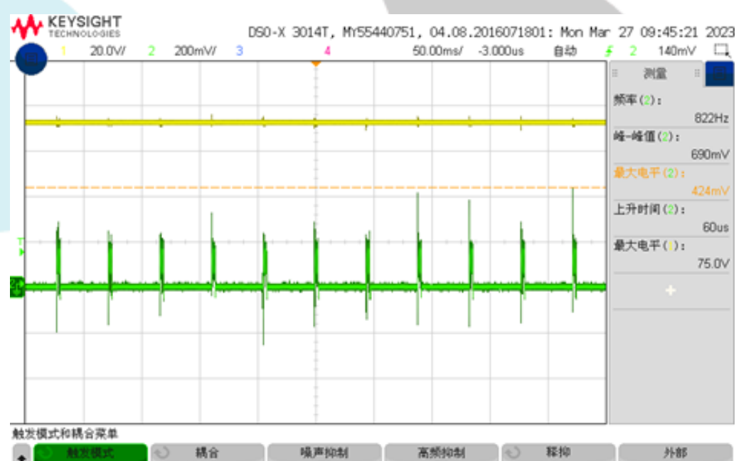
Figure 9, Short circuit & Output voltage
