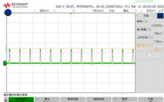
Figure 9, Short-circuit & Output voltage (I out = 40A)
