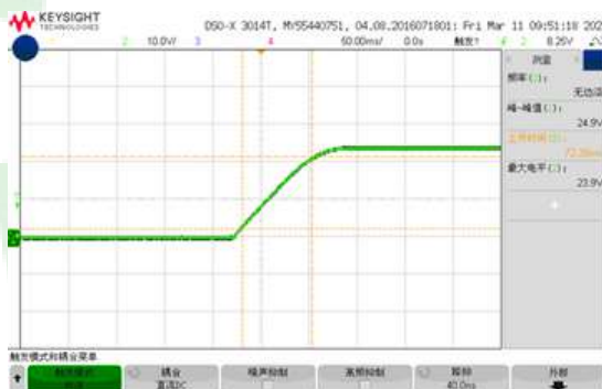
Figure 6, Output voltage established (I out = 40A)
