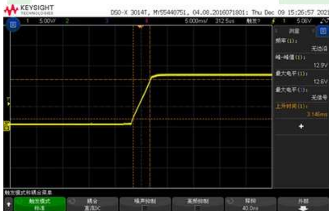
Figure 6, Output voltage established (Iout = 1A)
