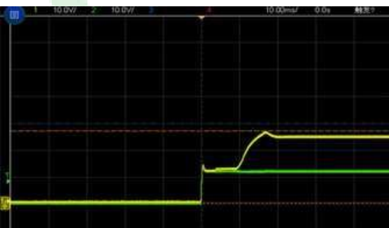
Figure 6, Output voltage established ( I_{out} = 5\text{A} )
