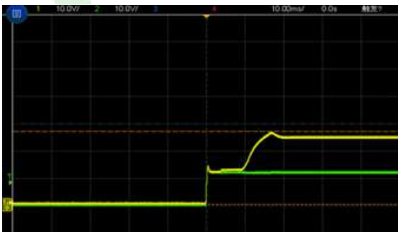
Figure 6, Output voltage established ( I_{out} = 5\text{A} )
