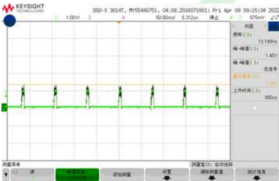
Figure 9, Short-circuit & Output voltage (Iout = 60A)
