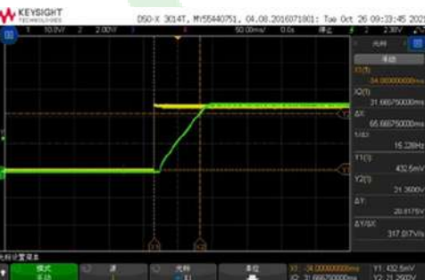
Figure 8, Boot delay time
