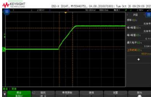
Figure 6, Output voltage established (Iout = 15A)
