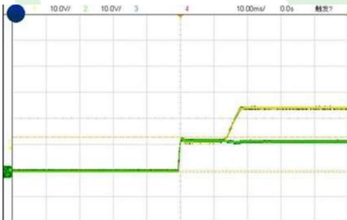
Figure 6, Output voltage established ( I_{out} = 10\text{A} )
