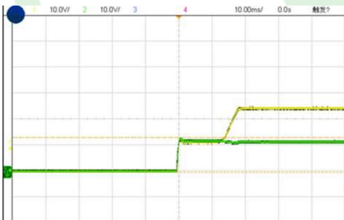
Figure 6, Output voltage established ( I_{out} = 10\text{A} )
