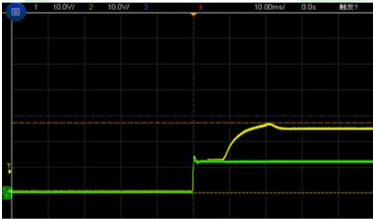
Figure 6, Output voltage established ( I_{out} = 1\text{A} )
