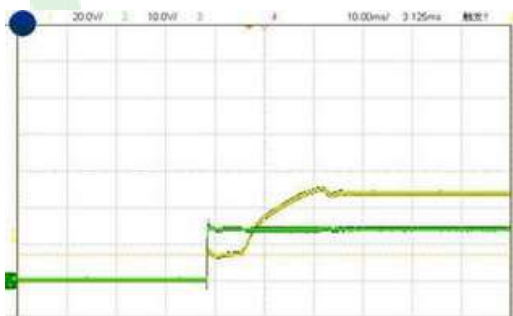
Figure 6, Output voltage established ( I_{out} = 2\text{A} )
