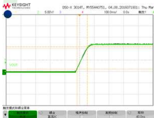
Figure 6, Output voltage established ( I_{out} = 60\text{A} )
