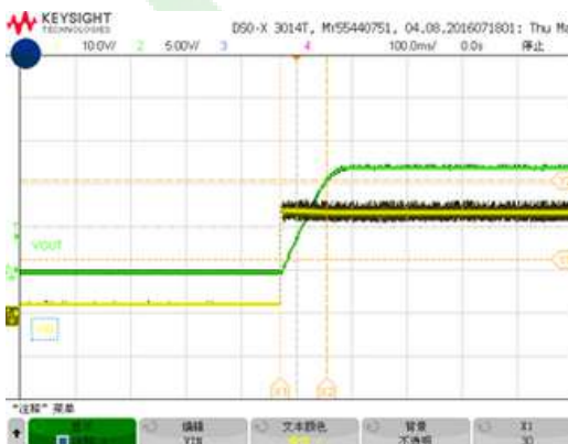
Figure 8, Boot delay time ( I_{out} = 60\text{A} )
