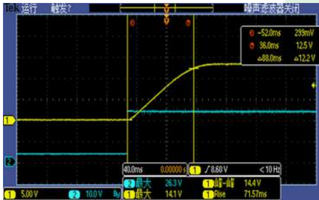
Figure 6, Output voltage established (Iout = 20A)
