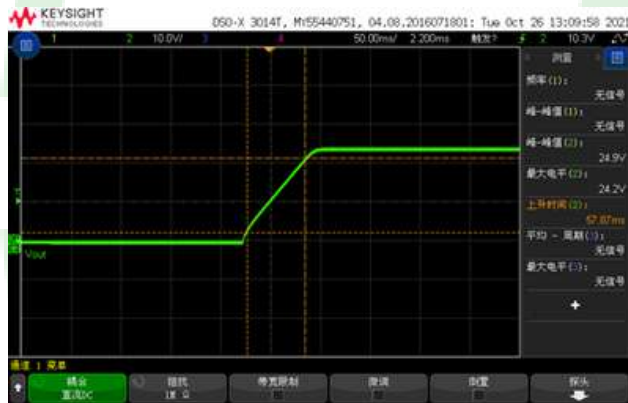
Figure 6, Output voltage established ( I_{out} = 10\text{A} )
