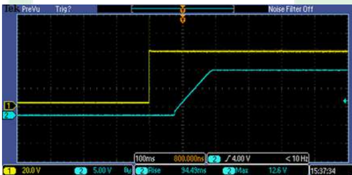
Figure 6, Output voltage established ( I_{out} = 10\text{A} )
