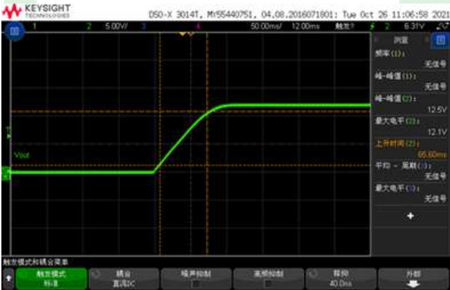
Figure 6, Output voltage established (Iout = 20A)
