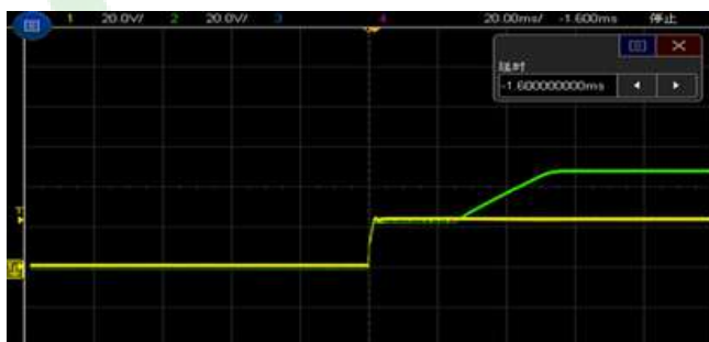
Figure 6, Output voltage established ( I_{out} = 10\text{A} )
