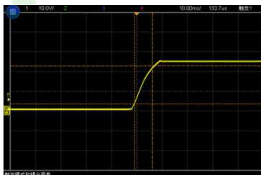
Figure 6, Output voltage established ( I_{out} = 6\text{A} )
