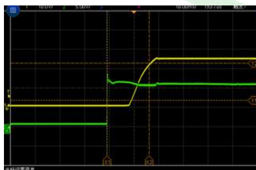
Figure 8, Boot delay time
