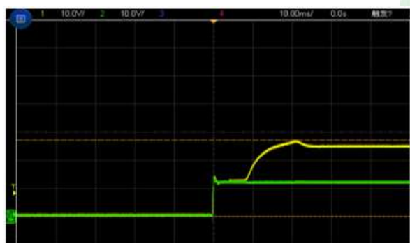
Figure 6, Output voltage established ( I_{out} = 20\text{A} )
